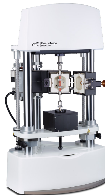
Figure 1. ElectroForce DMA 3200 instrument equipped with a forced-convection oven and tensile testing fixtures
