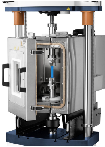
Figure 2. ElectroForce 3330 with oven and tensile fixture
