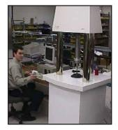
In order to properly characterize the heel tissue, an actuator had to be found that would provide the fast rate 'ramp and hold' protocol required of the viscoelastic soft tissue model. The model assumes that no relaxation occurs during the ramp portion of the testing. The worst case scenario is a displacement of 15 mm in 20 to 25 ms.
