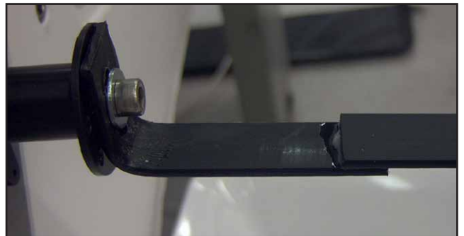
Single lap shear of tissue sample with fixture assembled
