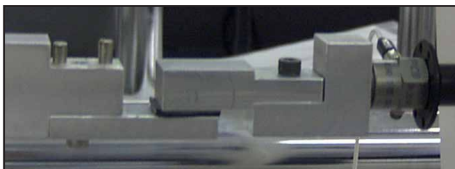
Single lap shear of uncured rubber
