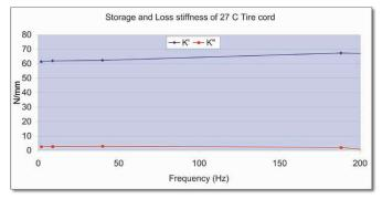
The modulus at 250°F was approximately 50% of the modulus at room temperature. The measured phase angle (tan delta) was the same at either temperature.
