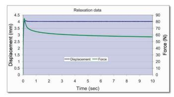
This test showed a reduction in force to 28.5 N per cord after 10 seconds. Level crossing data acquisition was used to optimize the data file size for this test.
