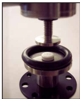
ODT mounted onto test platen before loading.
