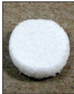
Figure 1 – The degradation of a disc PLGA scaffold was investigated under dynamic loading conditions.
