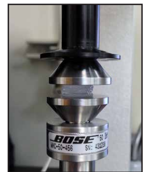
Figure 3 - Specimen Loaded Between Compression Platens
