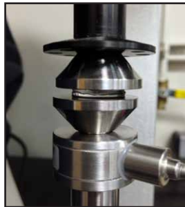
Figure 5 - Hydrogel Specimens Loaded Between Compression Platens
