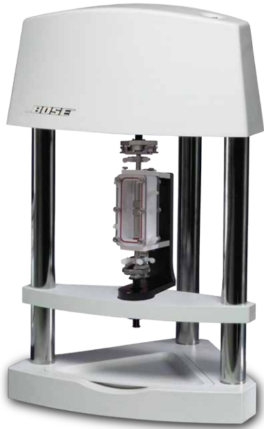
A BioDynamic chamber can be added to the ElectroForce 3200 Biomaterials test instrument to apply compressive (or tensile) loading on biological samples.
