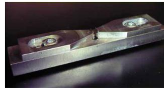
Figure 3. Bottom span of custom 4-point bend fixture.
