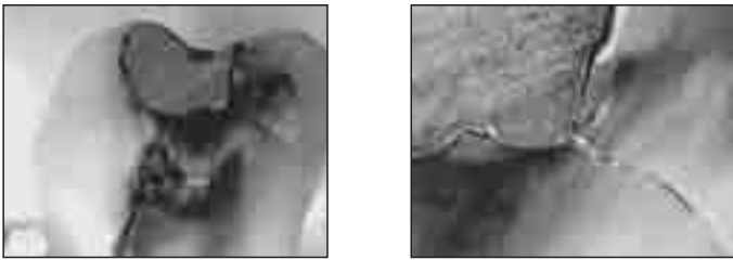
Tooth fractures originating at the boundary of a repair may indicate the presence of cyclic crack growth
