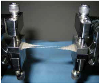
Figure 4. A PLGA test sample in the final pull to failure test.
