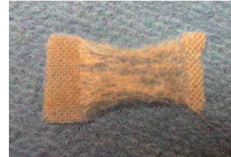
Figure 2. PLGA Sample after preconditioning cycles
