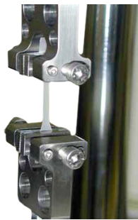
Figure 2. Tensile Specimen (ASTM D638 Type V)
