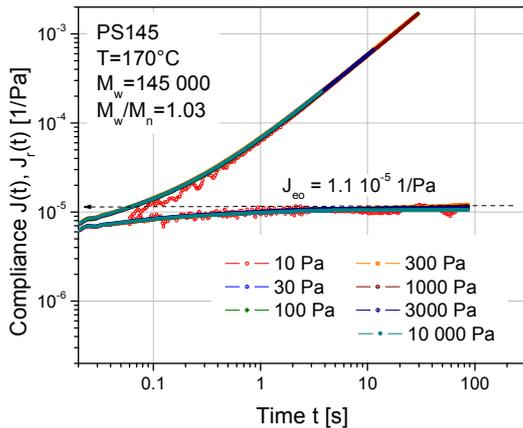
Figure 6: Creep Recovery of a narrow distributed PS145 over a stress range from 10 to 1000 Pa
