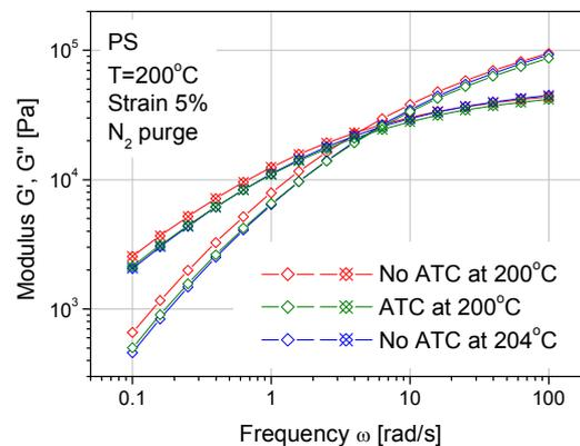
Figure 7: Frequency sweep performed with and without ATC. Without ATC, the a 4 °C temperature offset is needed to match the data obtained with ATC ON
