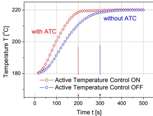
Figure 8: Temperature profile for a temperature step from 180 to 220°C with and ATC ON and OFF
