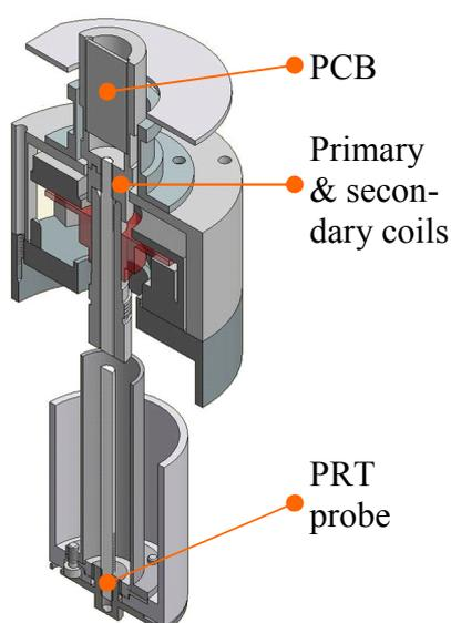
Figure 2: Upper test fixture for ETC with wireless temperature sensor ( for ATC
