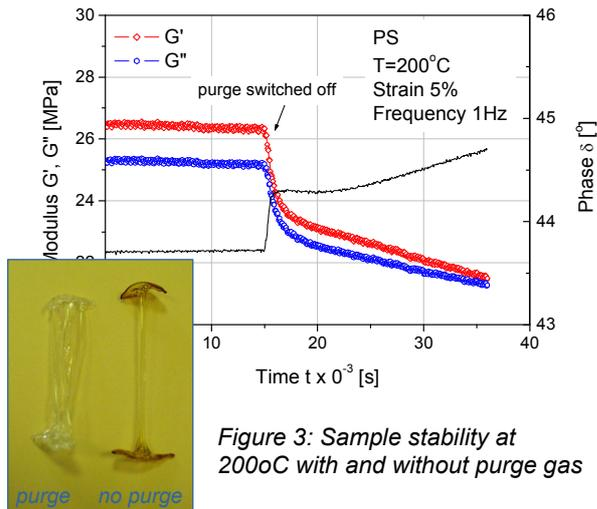
Figure 3: Sample stability at 200°C with and without purge gas
