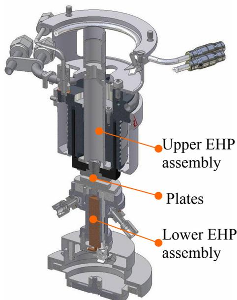
Figure 1: Schematics of the EHP for AR2000EX and AR-G2
