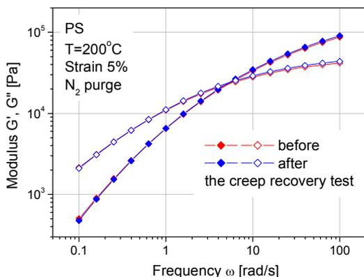
Figure 4: Frequency sweep before and after a 16 hour creep recovery test
