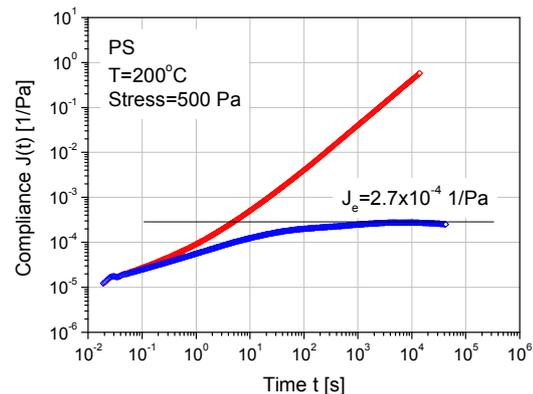
Figure 5: Creep Recovery test of the PSref at  $200^\circ\text{C}$ . Test time 16 hours
