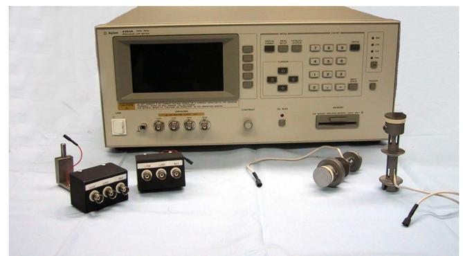
Figure 2: Dielectric option with HP bridge
