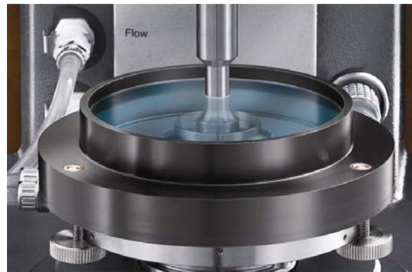
Figure 2: AR Rheometer Peltier plate immersion cell
