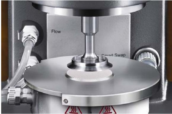
Figure 1: AR Rheometer with crosshatched geometry
