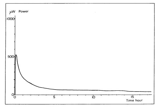
3. 0.012 g Lithium and 0.56 g Propylene Carbonate at 70°C. The components were sealed together in the same way as in experiment 2. The rate of heat production was much
