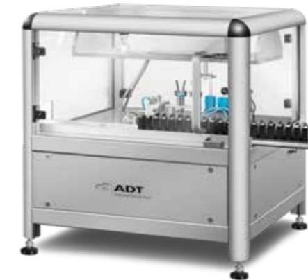
The finite difference method for density measurement relies on the measurement of sample weight dry, and immersed in a fluid, usually water. The difference between the dry and immersed weight is used with the known density of the fluid to calculate the volume of the specimen to a high degree of accuracy, irrespective of geometry.
