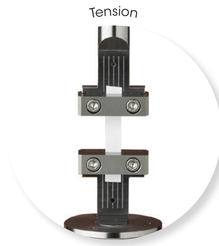
PET Film - Tension 50 µm thick
