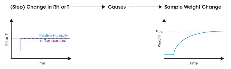
The recorded weight change rate over time is characteristic for the sorption kinetics. It indicates how fast humidity ad- or absorbs in the material or is released – desorbed – from the material. This is a characteristic property of the sample material. Weight changes can be fitted using TRIOS with an exponential model providing the time constant k of the sorption kinetics.
