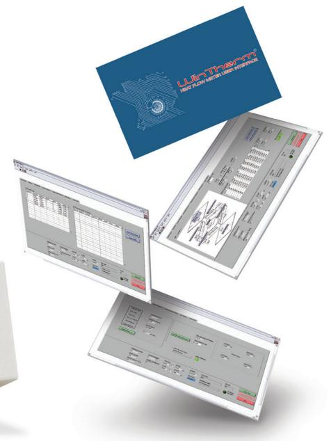
Accelerated testing - the average heat flow of the upper and lower heat flux sensors is calculated, and stabilizes much faster than individual signals. Accurate measurements (to within +/- 0.4%) can be made in less than half the time, increasing laboratory throughput.
