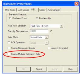
Once activated, the multiple calibration table can be viewed by selecting **Calibrate/Cell Temp Table** or by clicking on the Browse button (...) next to the new **Calibration Set** parameter on the Notes page of experimental setup, as shown in the figure below.
