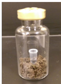
Picture 1. A 20 mL reaction vial with a solution of NaOH placed into the chamber for calorespiration determinations.
