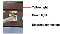
2 Connect one end of the Ethernet cable into the instrument's Ethernet port.
