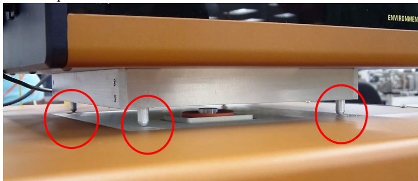
Figure 5 Pins on the bottom of the Environmental Module (EM-900 shown).
