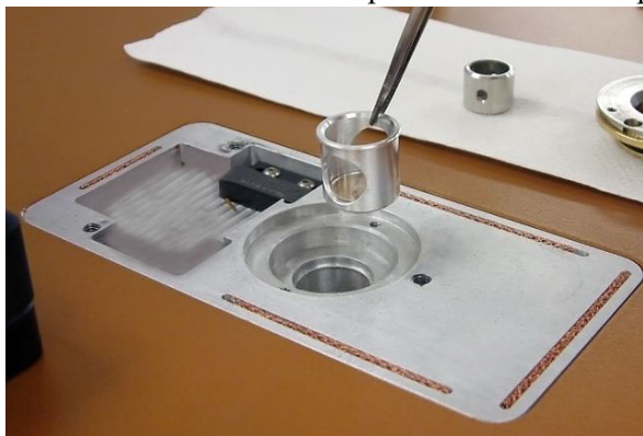
Figure 20 Extract and clean the optics.
