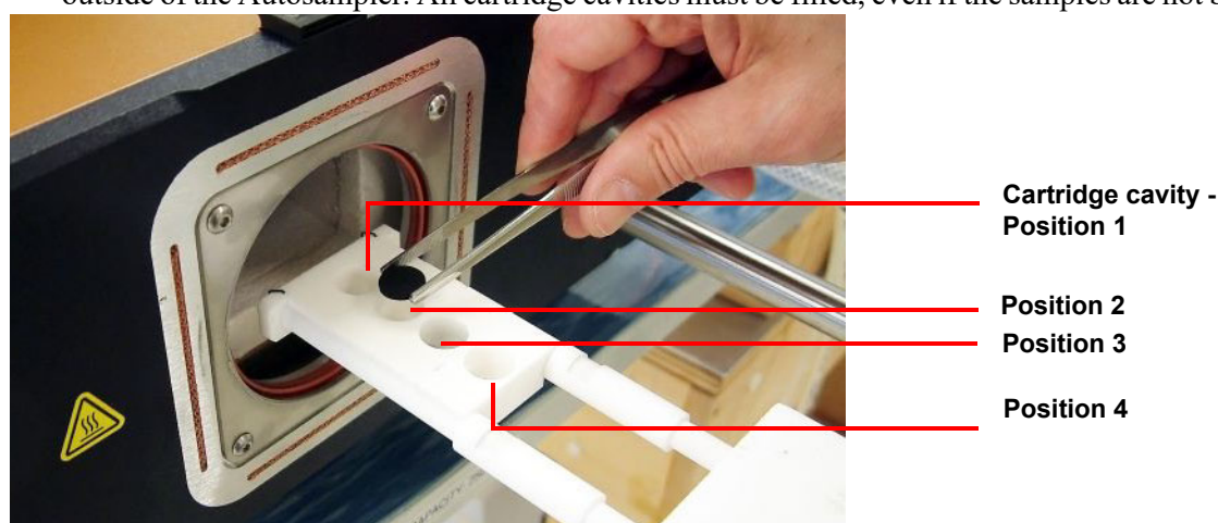
Figure 14 Loading the sample into a cartridge in Position 2.
