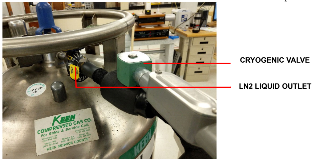
Figure 10 LN2 tank connections.
