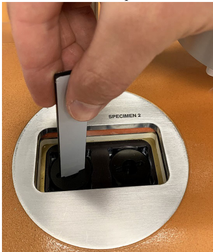
Figure 16 Removing the sample holder cover.
