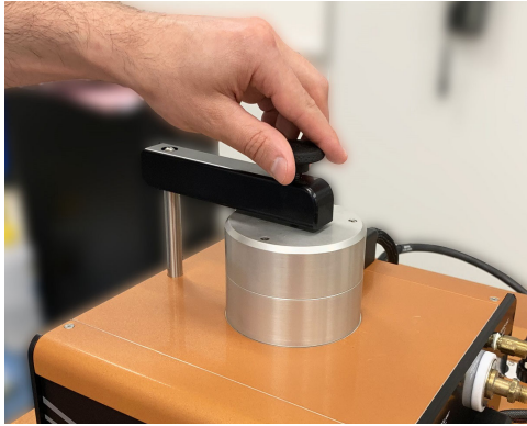
Figure 24 Unlocking the locking arm.
