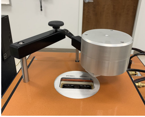
Figure 14 Swing the Solid State Detector away from the sample area.
