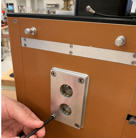
Figure 28 Remove the light pipe assembly.
