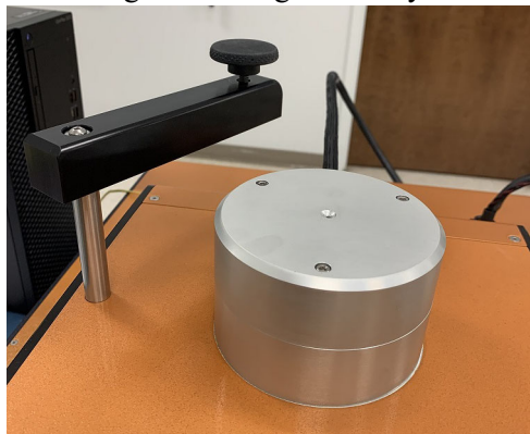
Figure 13 Swing the locking arm away from the Detector.
