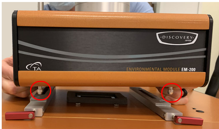
Figure 6 Pins on the bottom of the Environmental Module.
