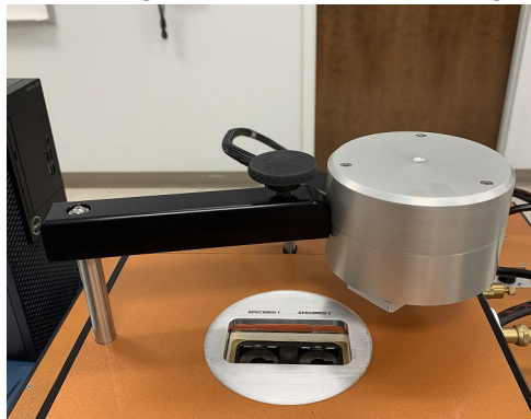
Figure 26 Locking arm holding the Solid State Detector in place.
