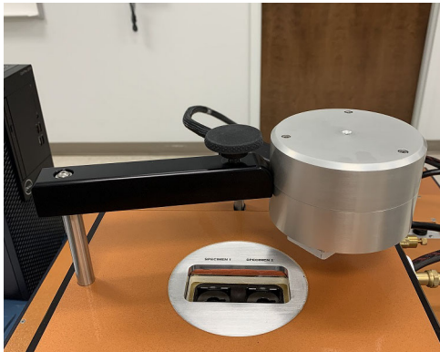
Figure 15 Locking arm holding the Solid State Detector away from the sample area.
