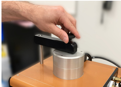
Figure 12 Unlocking the locking arm.
