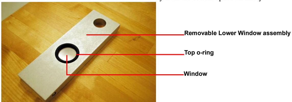
**Figure 42** Removable Lower Window assembly removed from bottom optics assembly.
