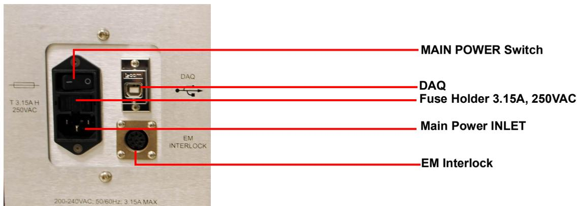
**Figure 8** DLF back panel connections.
