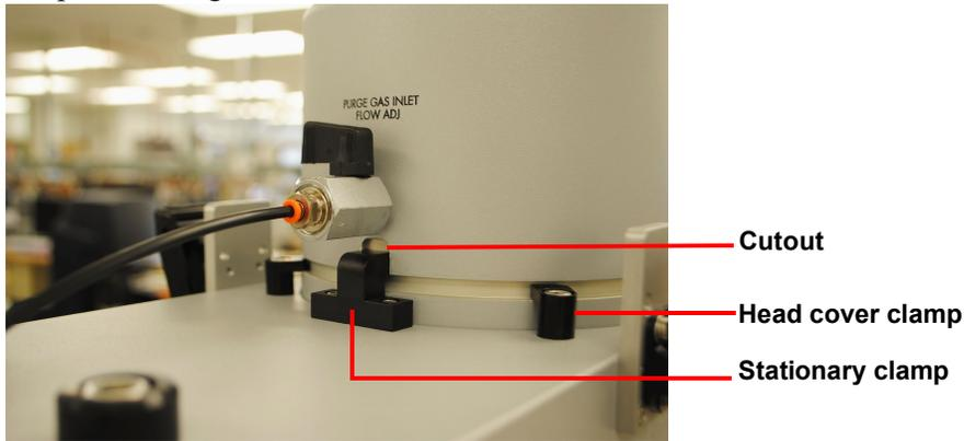
Figure 45 Cutout aligned with stationary clamp.
