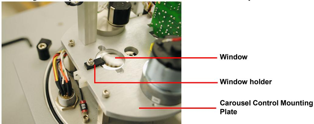
**Figure 44** Window holder securing the window in place.
