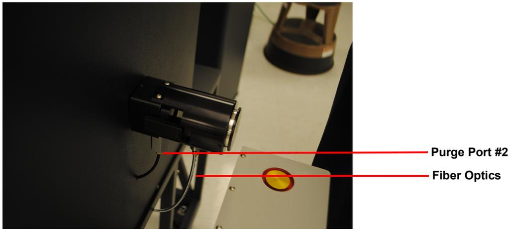
**Figure 12** Front purge port and Pyrometer fiber optics.
