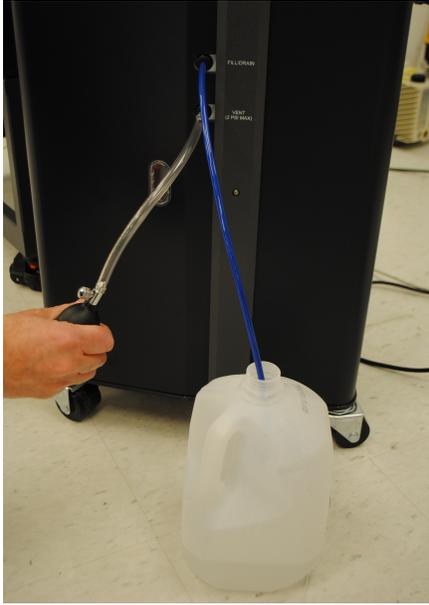
**Figure 52** Draining the fluid.
