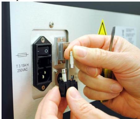
**Figure 49** Remove the fuses.
