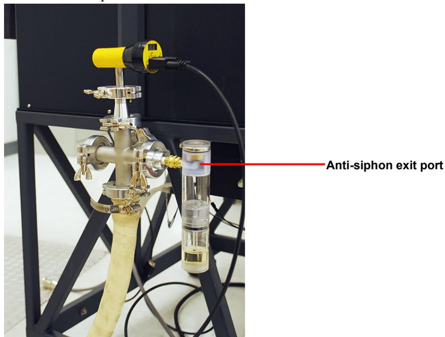
**Figure 26** Anti-siphon exit port attached to the EM-2800
