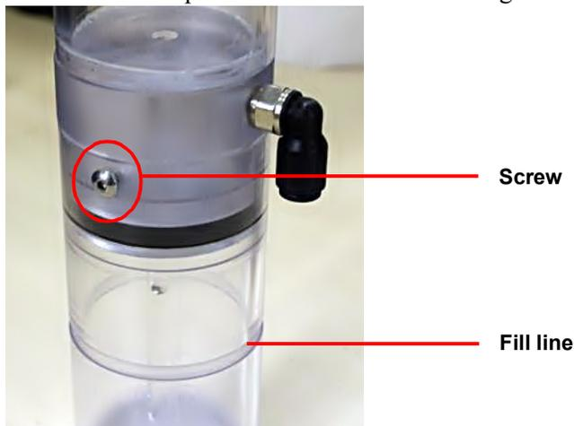
**Figure 25** Anti-siphon exit port screw and fill line.
