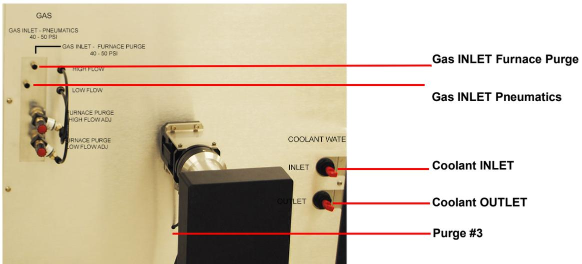
**Figure 11** Environmental Module-2800 back-right panel connections.
