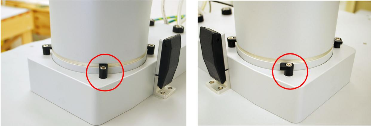
**Figure 43** head cover clamp securing the head (left); clamp turned away from the head (right).
