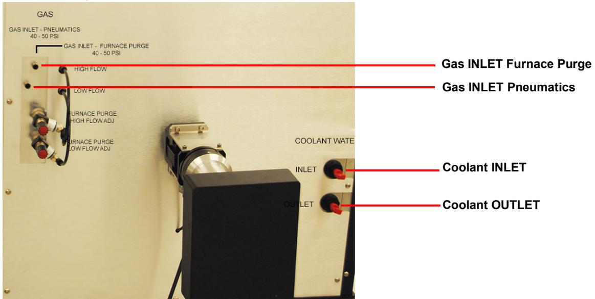
**Figure 27** Coolant and gas connections on the back of the EM.
