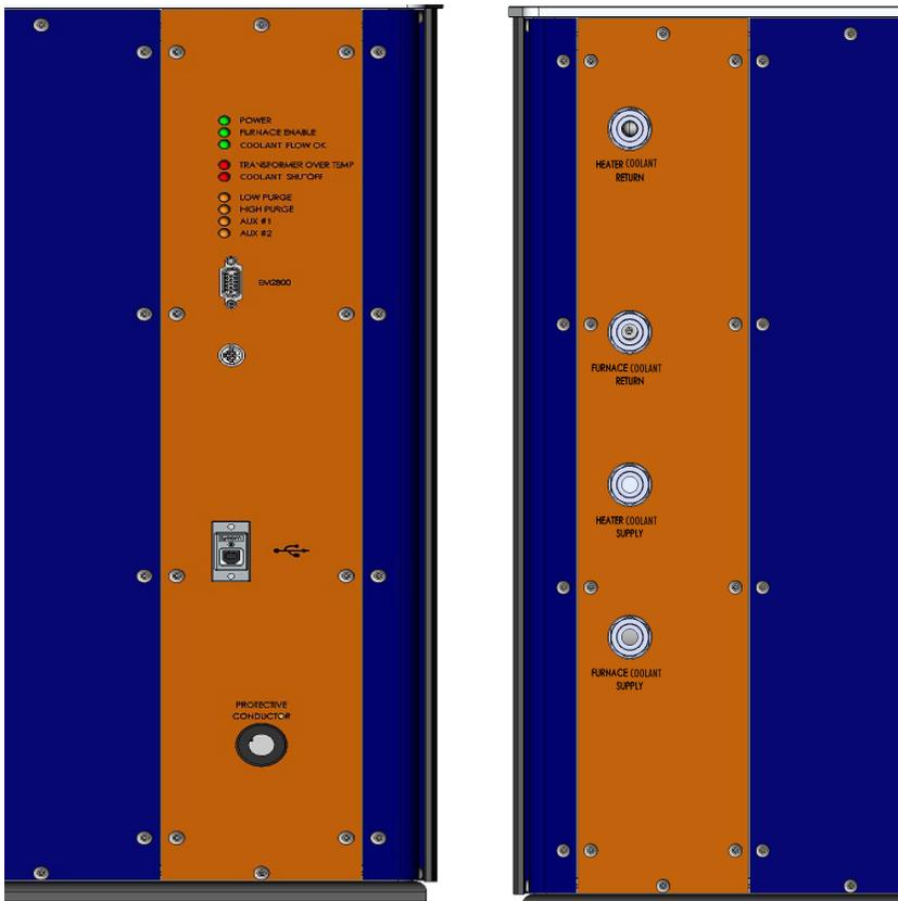
**Figure 21** Power Cart front panel electrical (left) and water (right) connections.
