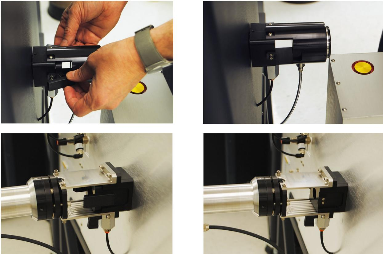
Figure 46 **Top left:** Unlatching the front pyrometer port; **Top right:** Window holder removed from front pyrometer port.
