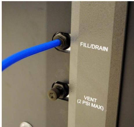
**Figure 50** Fill/Drain tube.
