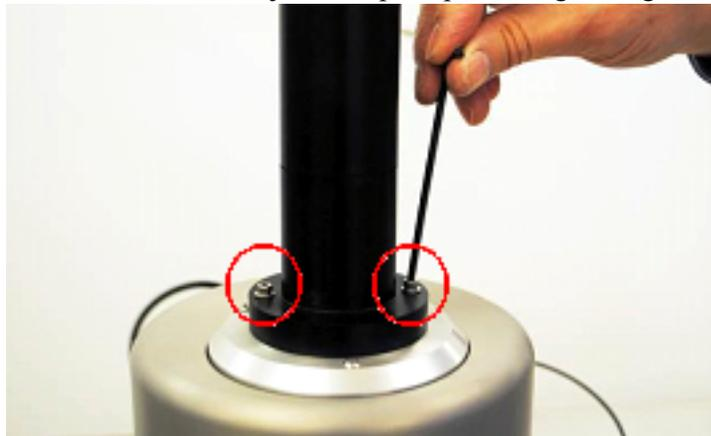
**Figure 20** Tighten EM-2800 wand screws
