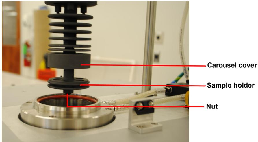
**Figure 16** Attach the samples holder.
