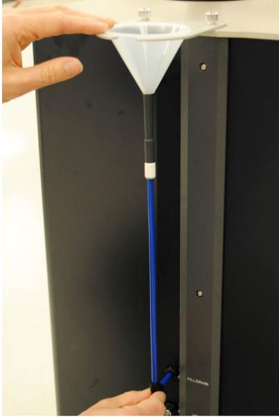
**Figure 54** Funnel and funnel tube on the DLF.
