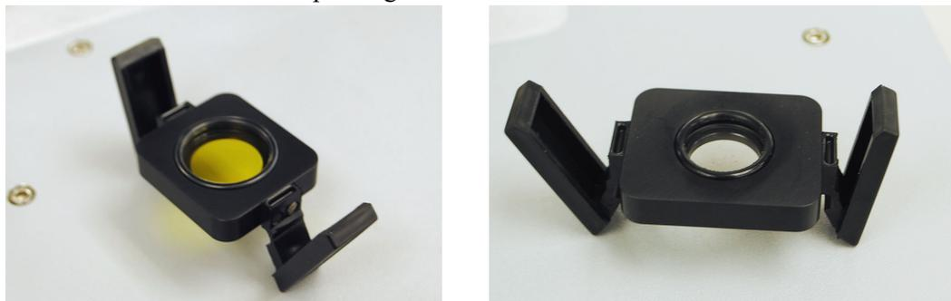
**Figure 47** Left: Back pyrometer port window holder; **Right:** Front pyrometer port window holder.
