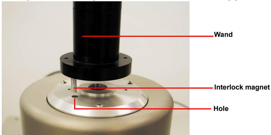
**Figure 19** Secure the wand to the EM-2800.
