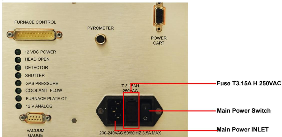
**Figure 10** Environmental Module-2800 IEC Panel connections.
