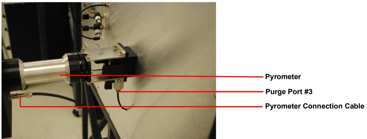
**Figure 13** Back purge port and pyrometer.
