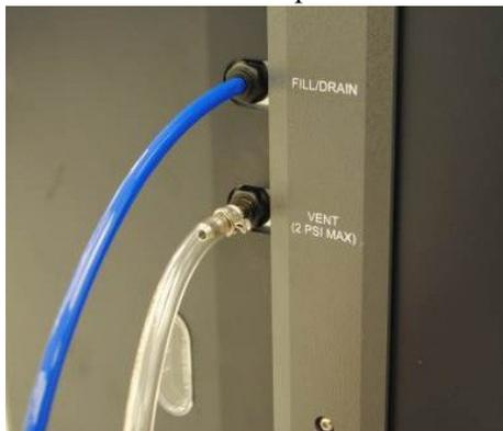
**Figure 51** Fill/Drain and Air Pump tubes connected.
