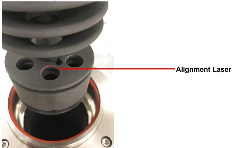
Figure 61 Alignment laser is on.
