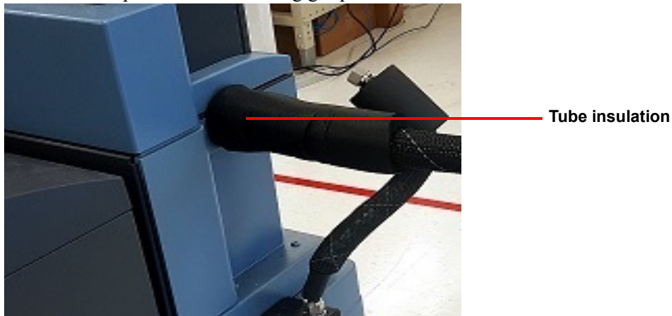
Figure 19 Tube insulation piece covering the Cooling Gas port and Cooling Gas tube.
