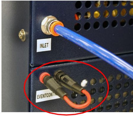
Figure 16 Remove jumper cable and retain for future use. .
