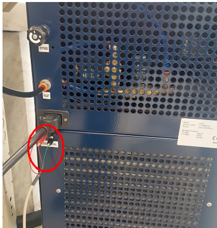
Figure 17 Left: Event cable connected to the ACS Event Control port; Right: Event cable connect to the Q800 Event Control port.
