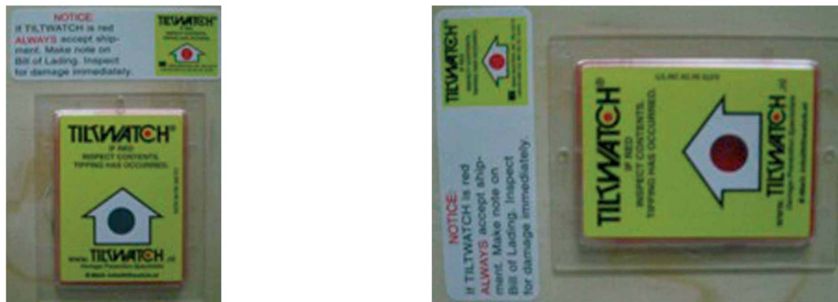
Figure 4 TiltWatch tilt sensor: Red not visible indicates normal handling (left); Red visible indicates potential mishandling.
