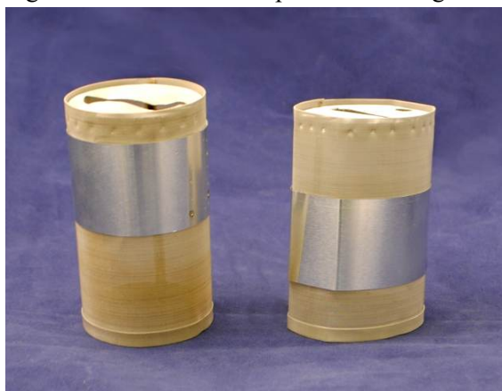
Figure 22 Left: Clamp screen for Film Tension; Right: Clamp screen for Cantilever and 3 Point Bending.
