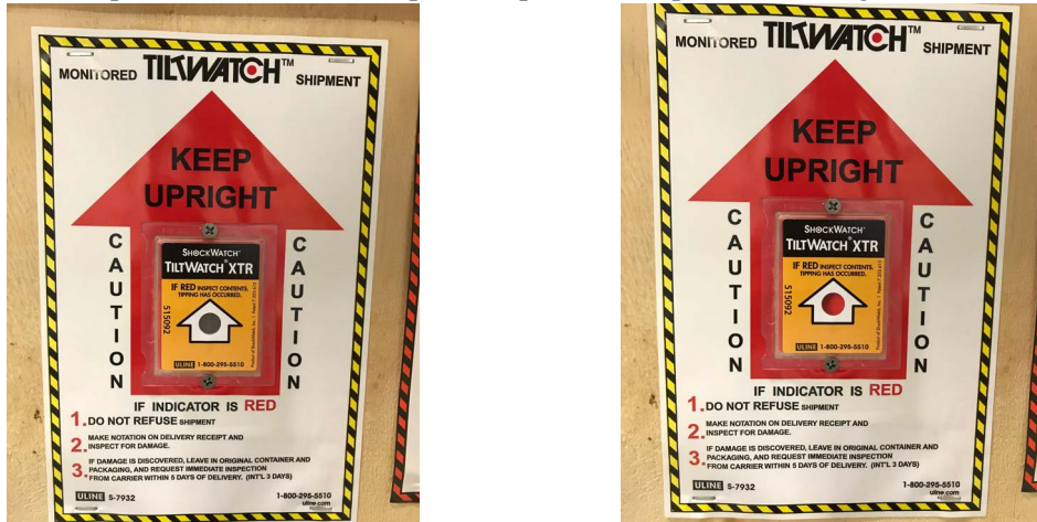
Figure 6 TiltWatch tilt sensor: Red not visible indicates normal handling (left); Red visible indicates potential mishandling (right).
