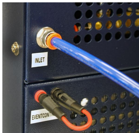
Figure 22 INLET port with Inlet tubing connected and Event Control port with jumper cable.
