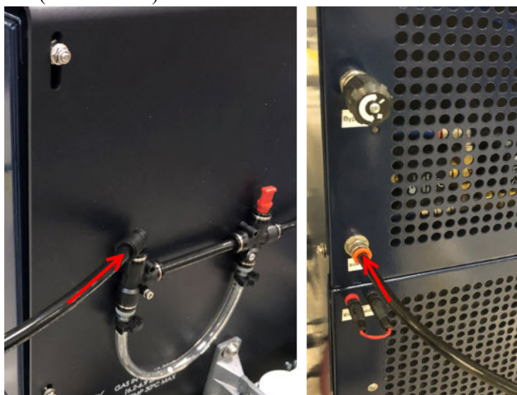
Figure 20 Flow indicator (left). Air INLET port (right) – SMC model.
