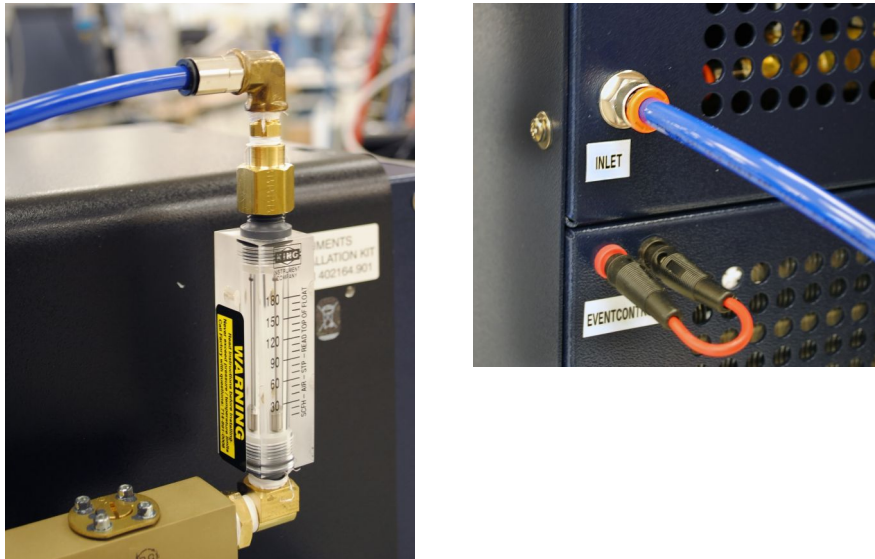
Figure 21 Flow indicator (left). Air INLET port (right) – Parker model (discontinued).
