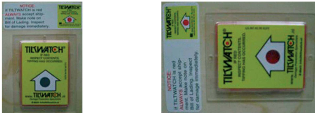
Figure 5 TiltWatch tilt sensor: Red not visible indicates normal handling (left); Red visible indicates potential mishandling (right).
