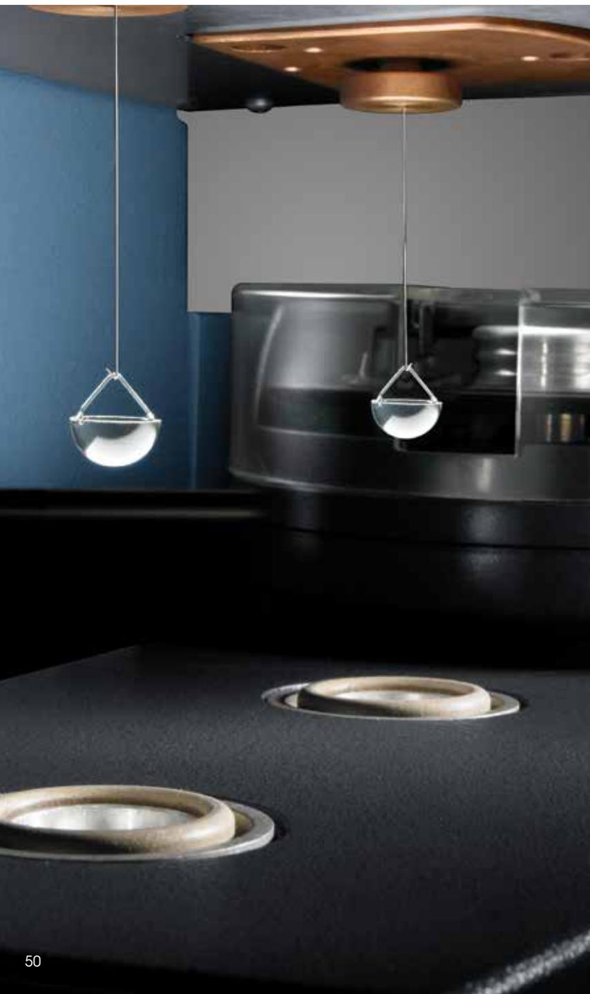
Vapor Sorption analysis is an established technique for determining the effect on materials of exposure to controlled conditions of temperature and humidity. Isotherm and Isohume™ experiments are the most commonly performed analyses.
