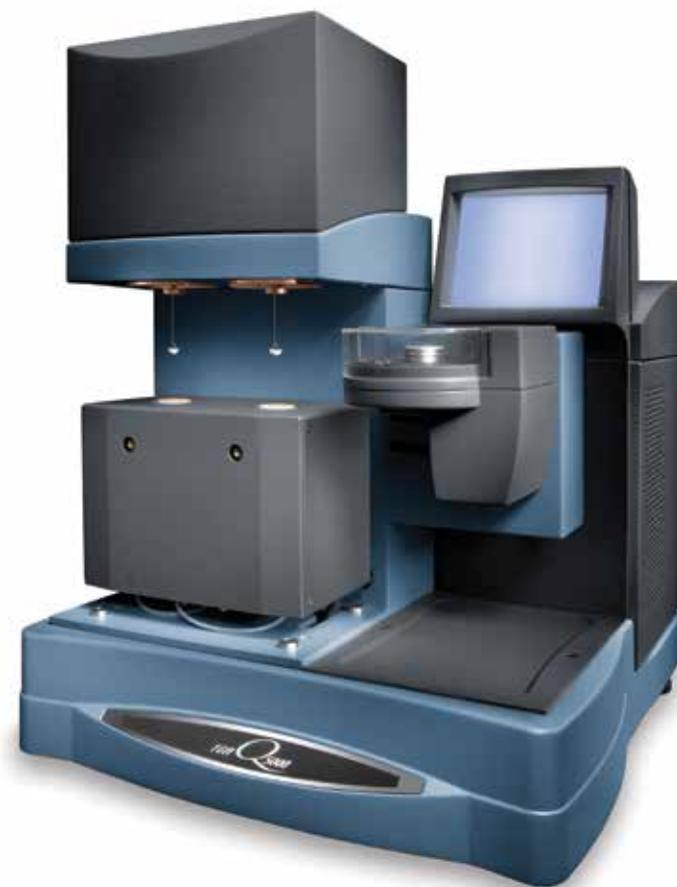
The Q5000 SA is a compact, benchtop instrument that delivers the performance and reliability required in a leading sorption analyzer designed for the study of materials under controlled conditions of temperature and relative humidity. Its modern, user-friendly design features a high sensitivity, temperature-controlled thermobalance, an innovative humidity generation system, a 10-position autosampler, and our latest Advantage™ software with Platinum™ features.
