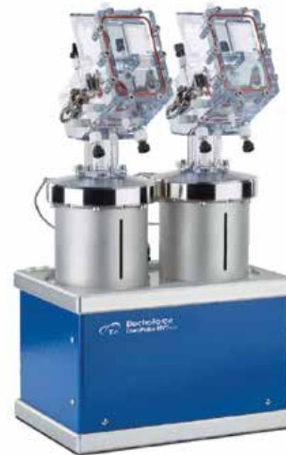
DuraPulse™ Heart Valve Test Instrument
