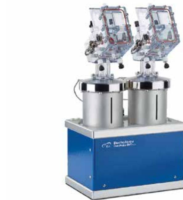
DuraPulse™ Heart Valve Test Instrument
