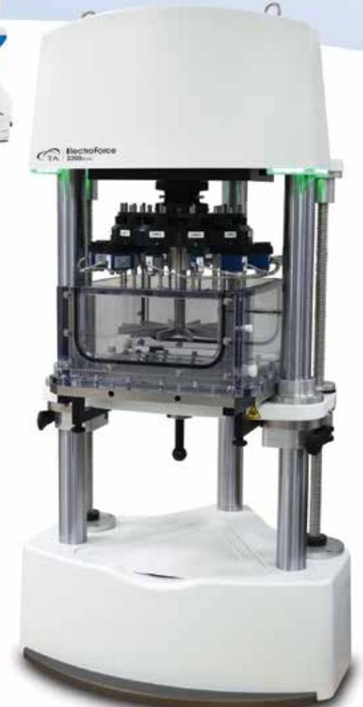
ElectroForce® Multi-Specimen Fatigue Testing Systems
