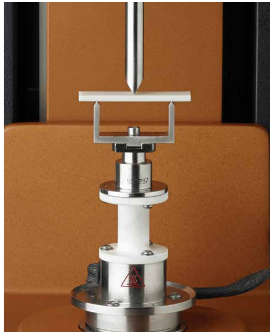
DMA Mode: DHR 3-Point Bending Clamp
