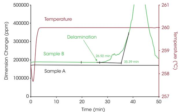
Figure 3. A Comparison of the Thermal Stability of Two Samples During Zone 3
