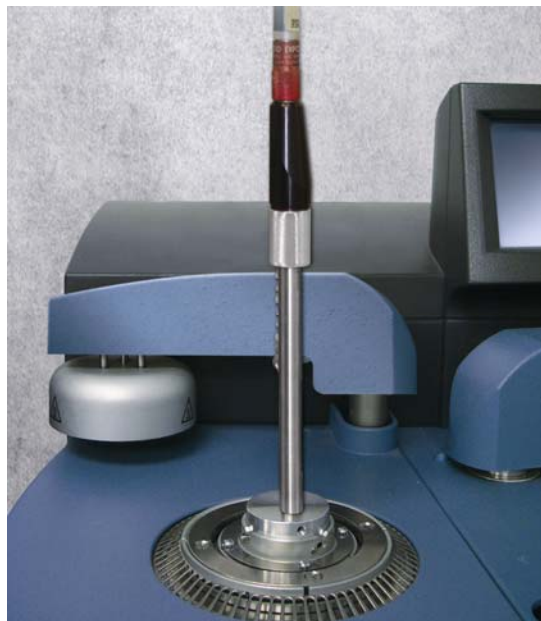
Figure 1. Raman Probe Interfaced to Q2000 DSC
