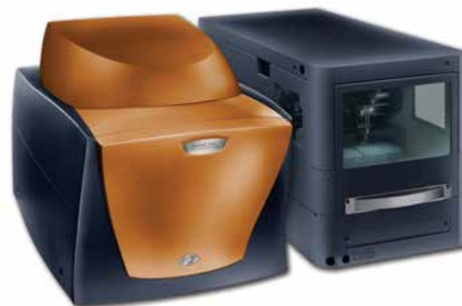
The Nano DSC is designed for ultra-sensitive measure of heat absorbed or released by dilute in-solution bio-molecules as they are heated or cooled. The capillary cell design, solid-state thermoelectric temperature control and easy cleaning ensure the highest sensitivity and data reproducibility for a wide variety of applications.
